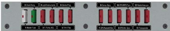
All the circuit breakers are labelled; additionally the placard shown below is applied inside the cockpit to give more detailed information. Here you can find detailed information about the rating of each CB.
