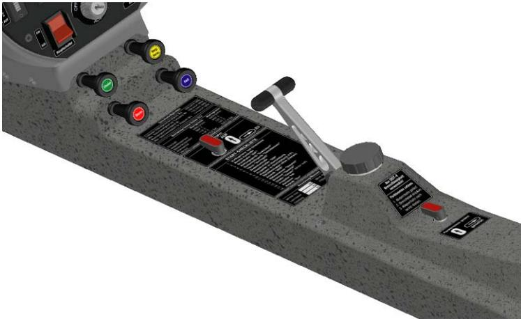
All controls are labeled. On the center console you will find all important placards, which post the operational limits for a safe operation of the aircraft. In addition a start-up checklist is provided.
