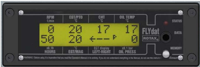
If any value approaches its limit, it starts blinking. If the limit is exceeded the red STATUS light will light up red.
